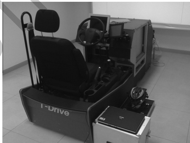
Fig. 1. Driving simulator: a car cockpit with steering wheel, accelerator–brake–clutch pedals, and gear lever. The scenario is projected on a 244 × 180 cm screen; the mean distance between participant and screen is 274 cm (depending on participant's height and seat style). A touchscreen for the secondary task is mounted to the right of the steering wheel; the distance between participant and touchscreen is approximately 75 cm.
