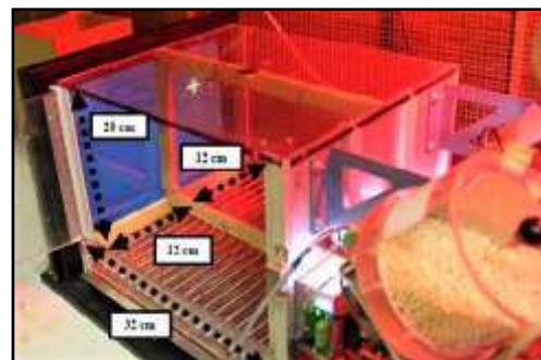
Figure 1. Interactive Rat Touch Screen Chamber (30.5×26.0 ×20.0) divided into two equal parts by the metal mesh. Each part of the chamber is adjusted for one animal and equipped with a pellet feeder and interactive sensory monitor.
