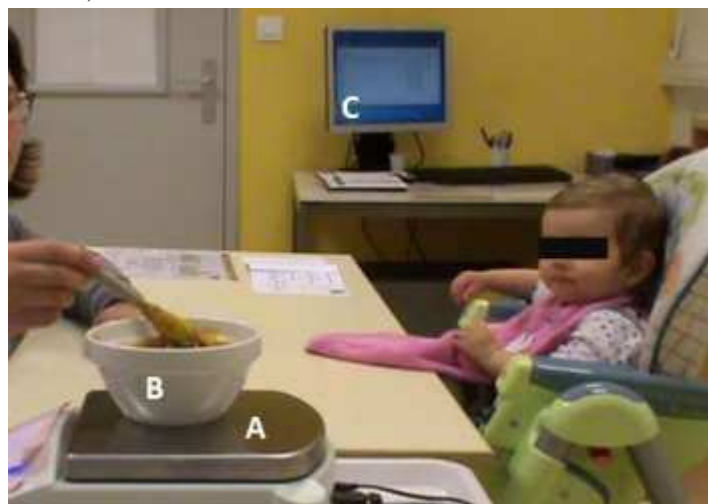
Figure 1. Recording device with the digital weighing scale (A), the bowl (B) and the computer (C).
