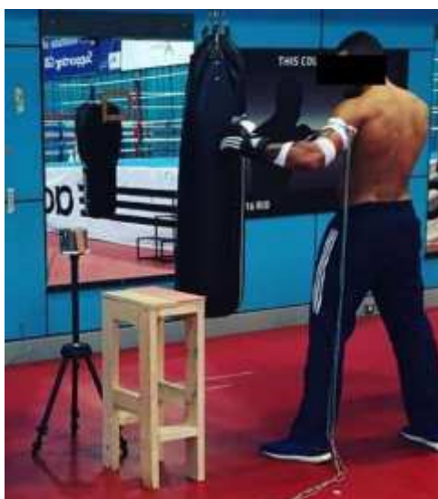
Figure 1. Field testing showing the Polhemus system set-up with one of the participants during the punch testing component of this study
